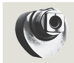
The heart-shaped cam and the linear drive mechanism which characterise all dormakaba cam-action door closers produce a rapidly decreasing opening torque, so greatly reducing the amount of effort required. This means that even children, the elderly and the disabled can open doors with ease. The user-friendliness of the system is further enhanced by the reliable latching action achieved by the fact that the closing force only rises in the end phase of the cycle.
