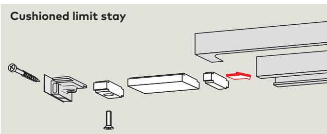
Cushioned limit stay simply slides into the slide channel. Adjustable between 80° and max. 120°. Also suitable for retrofitting. Fitting a cushioned limit stay prevents doors which are opened normally from impacting against adjacent walls.
