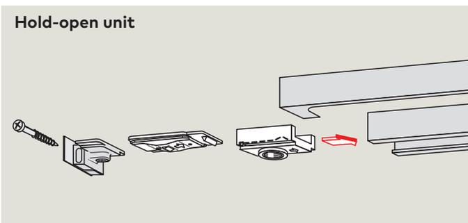
The **RF** mechanical hold-open unit ensures that doors are held open at precisely the correct angle – up to approx. 150° – without any fallback. The hold-open unit can be switched on and off by the user as required, and the pull-off force can be adjusted to suit each individual door situation. The RF hold-open unit is non-handed and can also be supplied for retrofitting to the slide channel at a later date.
