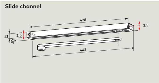
The **G-N** slide channel assembly comprises the main arm, slide channel, slide block, fixings, screws and end caps. The G-N slide channel is non-handed and can be combined with both door closers. Thanks to oblong holes in the fixing pads, it is possible to compensate for deviations in the drill hole pattern and to keep the door closer body and slide channel perfectly parallel.
